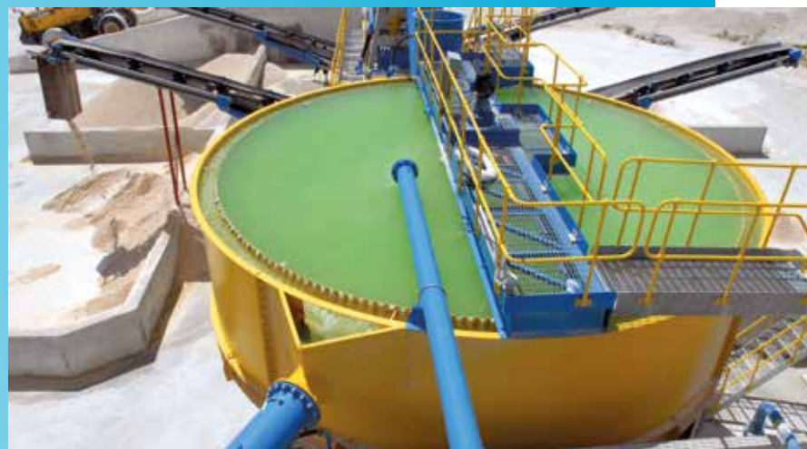
THE AQUACYCLE THICKENER RECYCLES UP TO 90% OF YOUR PROCESS WATER BACK TO YOUR PLANT.
